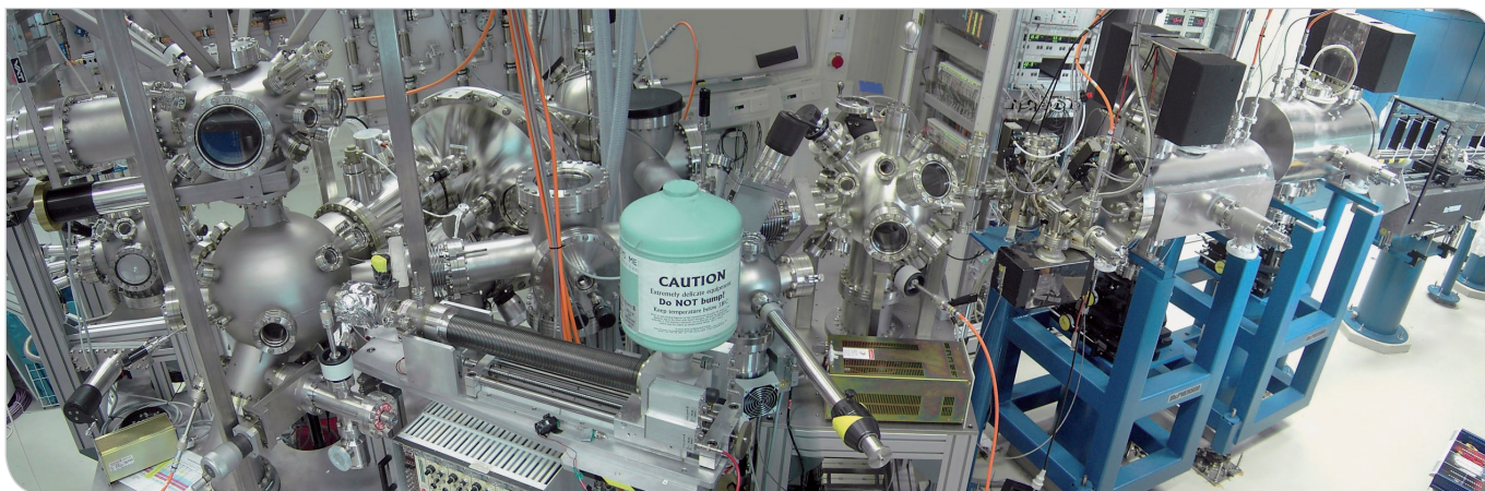
Fig. 1: Part of the cluster of experimental stations, preparation chambers, and loadlocks at WERA. The PEEM is located near the center.
