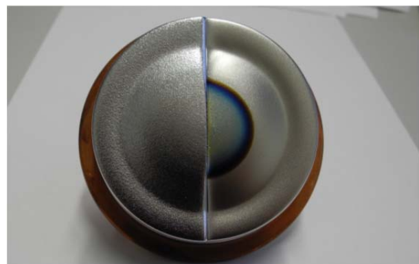
Fig. 2: Symmetrically divided Cr/Zr-target for the deposition of position-dependent \text{Cr}_x\text{Zr}_y\text{O}_z -films (diameter 75mm).
