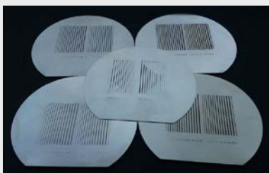
Figure 2: Five structured masks / thermoforming substrates used for microthermoforming experiments. The middle one is processed with cut through channels and holes.
