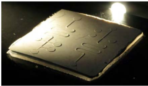
Fig. 4: Microfluidic chip replicated in ceramic feedstock on a polyethylene carrier layer.
