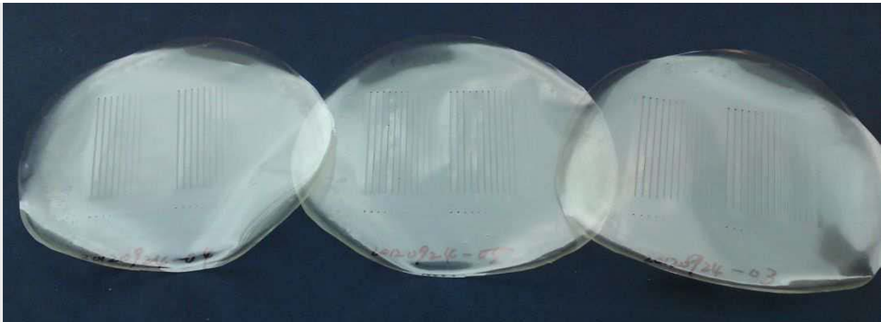
Figure 4: Three polycarbonate foils of 20 µm thickness which have been formed by microthermoforming into laser cut substrate.
