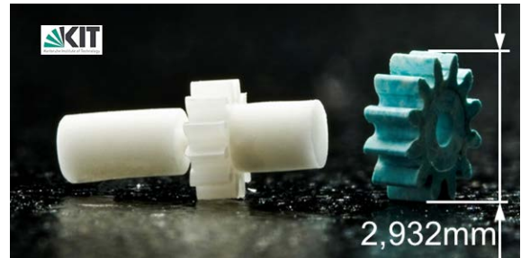
Fig. 4: Gear wheel/shaft sample made by two-component injection moulding of alumina (shaft) and zirconia ceramic (gear wheel). Combined sintered part (left) and green body (right).
