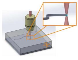
Sketch of the writing of a line in 3D-space inside a resist layer. The inset shows the modification in the voxel (blue) at the focal position. Only in the voxel two-photon absorption occurs.
