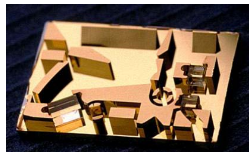
Fig. 4: Microoptical bench with cylindrical mirrors and fixing structures
