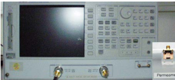
The high frequency permeameter consists of a strip-line measuring head on an attached vector network analyzer
