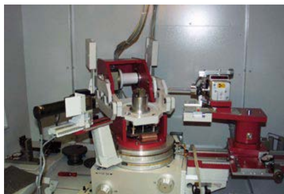
4 circle goniometer for XRD characterization (Seifert 3003 HR)
