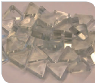
Prism demonstrators made of different transparent thermoplastics (PMMA, PMMI, PC) including composites filled with nanoparticles
