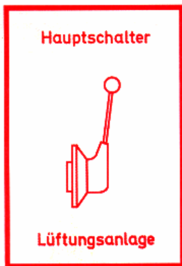
Master switch of electric equipment (e.g. ventilation system*)
