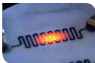
Laser modified cordierite: heating element (width 300 \mu\text{m} ) made of tungsten
