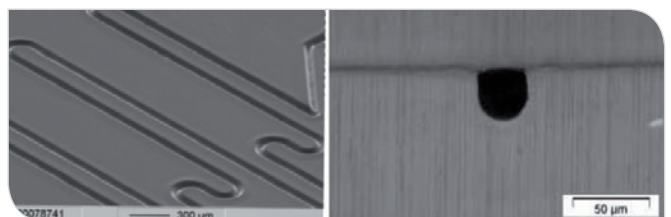
Laser structured fluidic chip (left) and cross section (right) of laser welded microchannel
