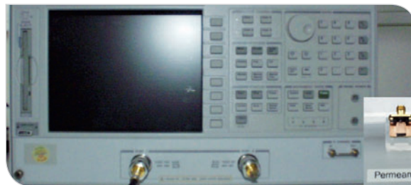
The high frequency permeameter consists of a coplanar measuring head on an attached vector network analyzer
