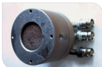
Retarding field analyzer for measurement of plasma potential, ion energy and energy distribution ions
