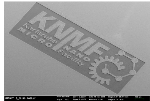
Fig. 1: Detail of an intermediate XRL mask (gold absorber height: 2.2 \mu\text{m} )
